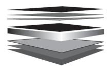
Finish Coat (Nominal 20µm) (Refer Notes 4 & 5) Universal Corrosion Inhibitive Primer (Nominal 5µm) **Conversion Coating**
